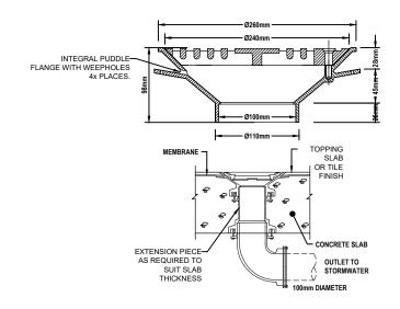
**FLOOR WASTE OUTLET DETAIL** NOT TO SCALE
