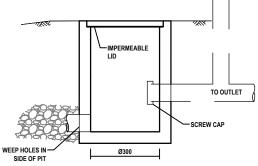
FIRST FLUSH WATER **DIVERTER DETAIL** N.T.S.
